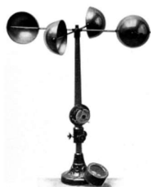
THE ROBINSON ANEMOMETER.
